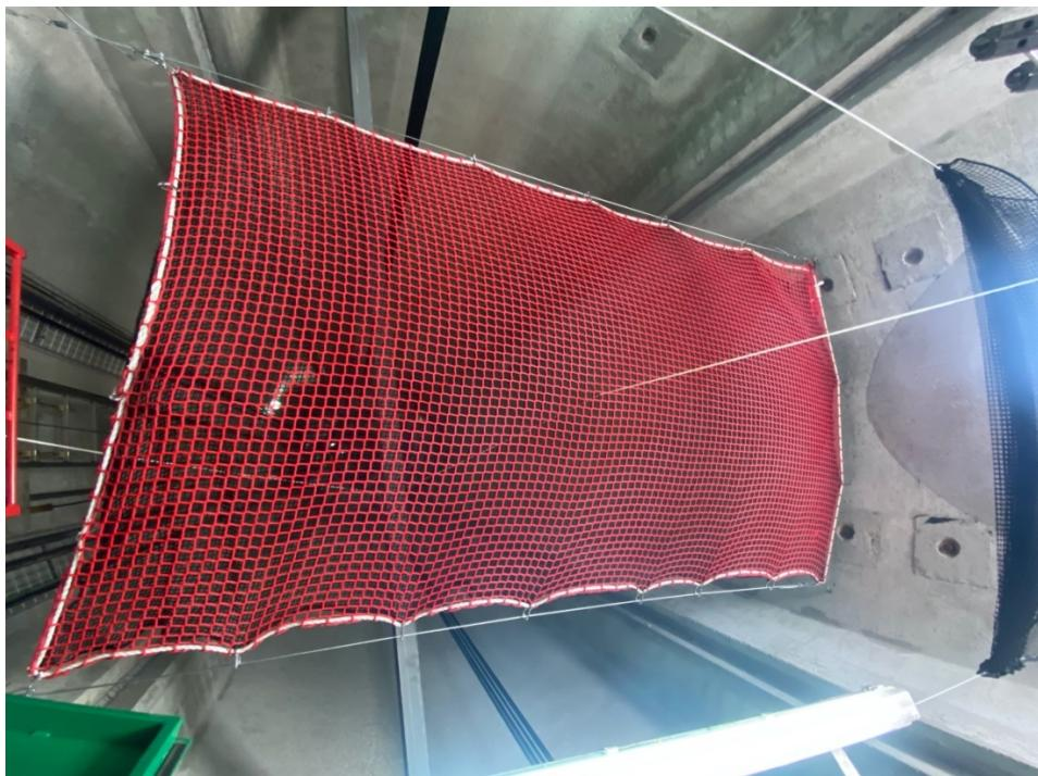
Imagen after the impact of the weight of 5 kg from 40 meters high
